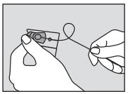
Straighten the lead wire.
